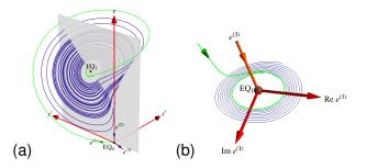
(a) Lorenz attractor plotted in [x', y', z], the doubled-polar angle coordinates, with points related by  $\pi$ -rotation in the [x, y] plane identified. Stable eigenvectors of  $EQ_0$ :  $\mathbf{e}^{(3)}$  and  $\mathbf{e}^{(2)}$ , along the *z* axis. Unstable manifold orbit  $W^u(EQ_0)$  (green) is a continuation of the unstable  $\mathbf{e}^{(1)}$  of  $EQ_0$ .
