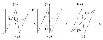
(a) boundary fixed point  $\overline{C}$ , asymmetric fixed points pair  $\{\overline{L}, \overline{R}\}$ (b) symmetric 2-cycle  $\overline{LR}$ (c) asymmetric 2-cycles pair  $\{\overline{LC}, \overline{CR}\}$  **Asymmetric cycles:** *R* generates a reflection of the orbit with the same number of points and the same stability properties
