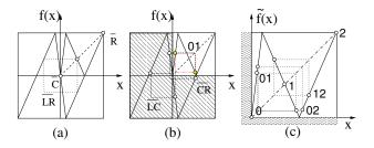
sawtooth map with the  $D_1$  symmetry f(-x) = -f(x) restricted to the fundamental domain. f(x) is indicated by the thin line, and fundamental domain map  $\tilde{f}(\tilde{x})$  by the thick line.
