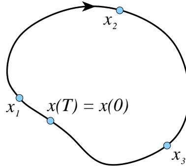
**Figure 2.3:** A periodic point returns to the initial point after a finite time,  $x = f^{T_p}(x)$ . Periodic orbit  $p$  is the set of periodic points  $p = \mathcal{M}_p = \{x_1, x_2, \dots\}$  swept out by the trajectory of any one of them in the finite time  $T_p$ .
