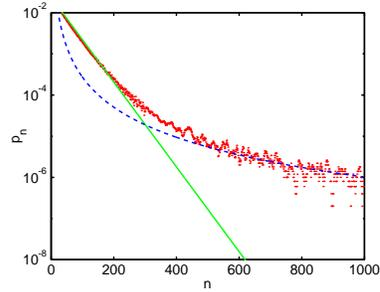
We see that, asymptotically, the escape from an intermittent repeller is described by power law decay rather than the exponential decay we are familiar with for hyperbolic maps; a numerical simulation of the power-law escape from an intermittent repeller is shown in figure 24.6.
