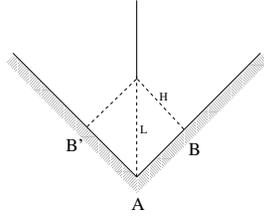
**Figure 38.4:** The billiard considered here. The dynamics consists of free motion followed by specular reflections off the faces. The top vertex induces diffraction while the bottom one is a right angle and induces two specular geometric reflections.
