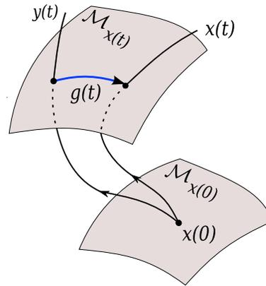
**Figure 13.1:** The freedom to pick a moving frame: A point  $x$  on the full state space trajectory  $x(t)$  is equivalent up to a group rotation  $g(t)$  to the point  $\hat{x}$  on the curve  $\hat{x}(t)$  if the two points belong to the same group orbit  $\mathcal{M}_x$ , see (12.2).
