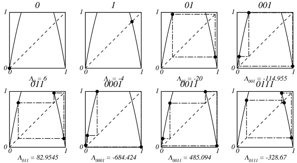
Figure K.4: Periodic orbits and stabilities for the logistics equation  $x_{n+1} = 6x_n(1 - x_n)$ .
